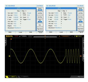
APM high performance AC source LIST function not only provides multiple waveform edition modes to modify all kind of power interference but also could realize transient transform between AC and DC. Via LIST edit, transform from AC to DC could happen in 90° degree of sine wave. It only need to set start angle in 90°. This kind of setting is flexible; we could set transform from AC to DC happen in positive peak of AC waveform which will be No-slot joint. It could improve power efficiency.
